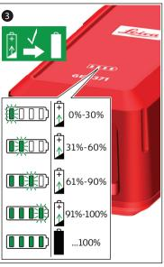
Battery Power Supply (with Power Cable)
